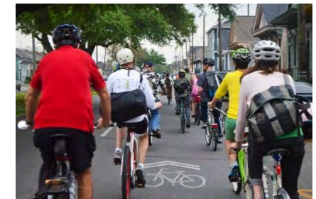
Sharrows pavement markings.
